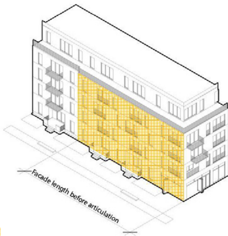
Figure 2-9 Facade length before articulation
