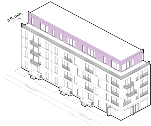
Figure 2-4 Height: 8-foot stepback above 4 stories
