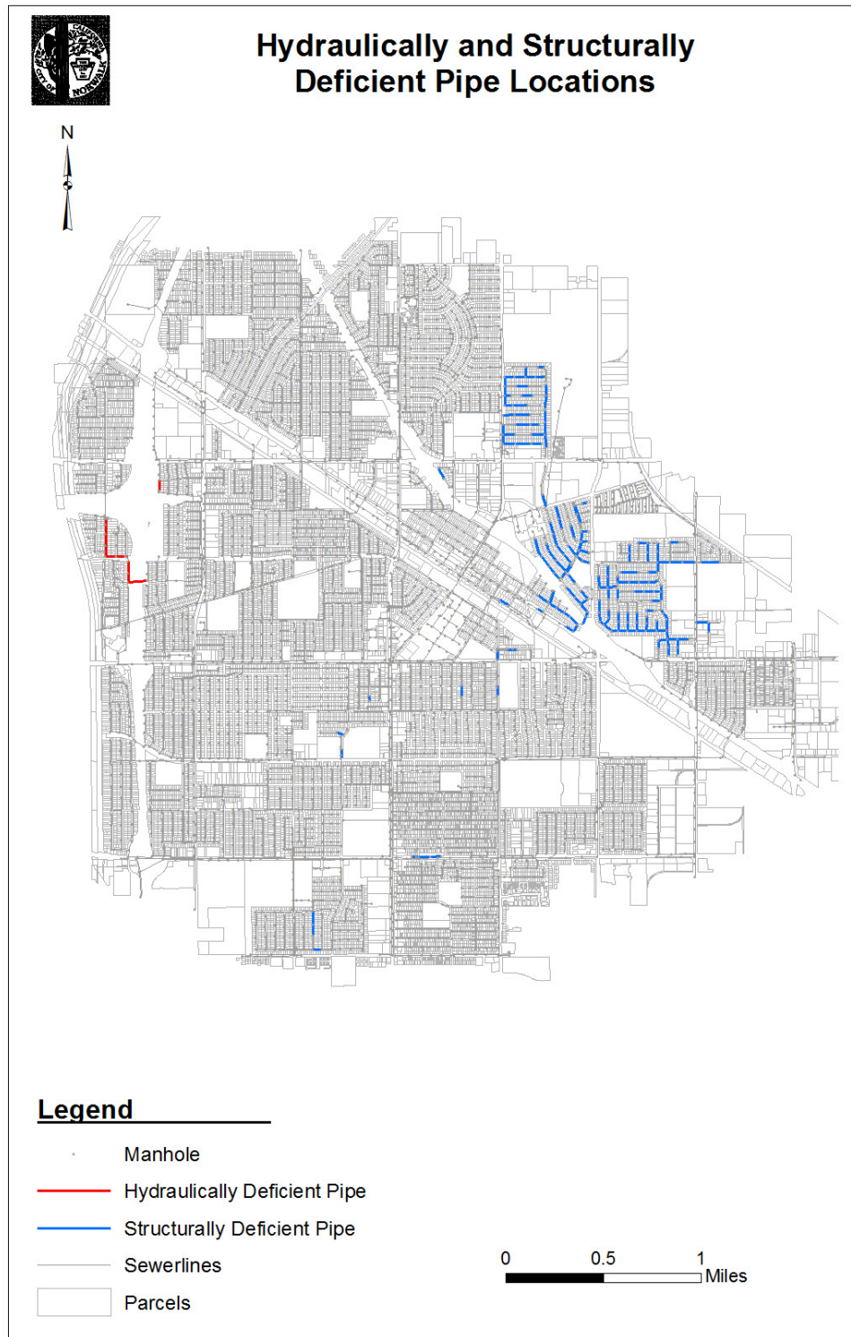
Exhibit 6-3 Hydraulically and Structurally Deficient Line Segments
