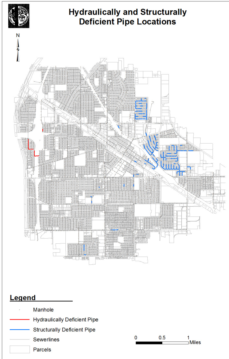
Exhibit 7-1 Hydraulically and Structurally Deficient Line Segments
