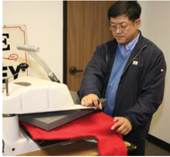
Mr. Khym gives an example of his heat press machine, transferring a sublimated image.
